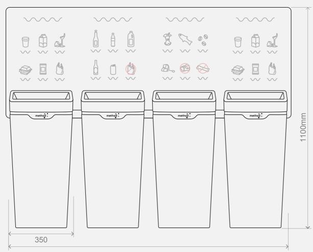
1560mm - 4 bins connected with HD connectors
